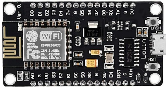
Figure 3.5: Microcontroller ESP8266 NodeMCU
