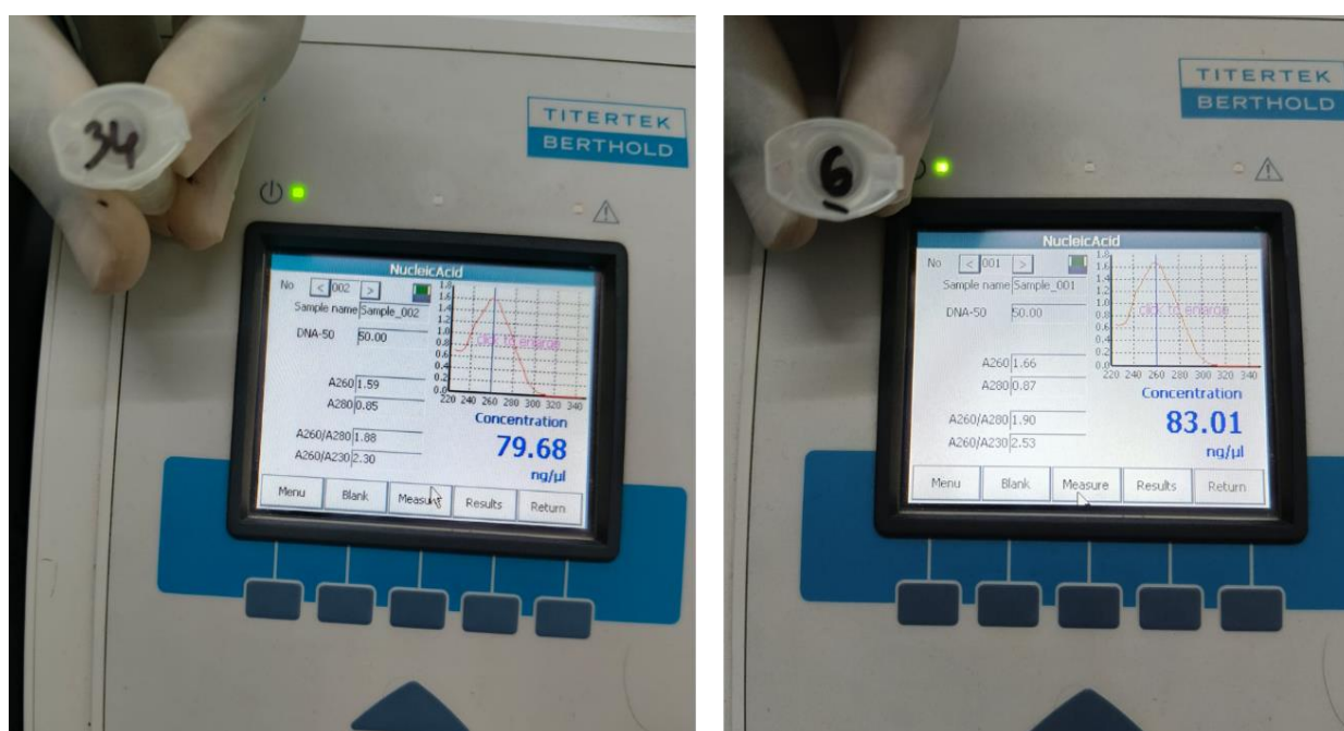
Figure 2.5: DNA concentration and purity measurement of the extracted DNA.
